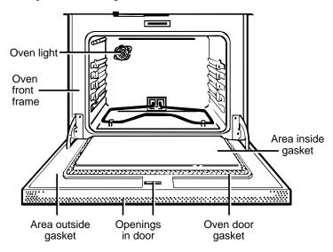
3. Clean spatters or soil on the oven front frame and the oven door outside the gasket with a dampened cloth. The oven front frame and the oven door outside the gasket do not get cleaned by the self-clean cycle. On these areas, use detergent and hot water or a soap-filled steel wool pad. Rinse well with a vinegar and water solution. This will help prevent a brown residue from forming when the oven is heated. Buff these areas with a dry cloth. Do not clean the gasket.
